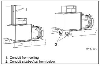
Figure 7-3 Typical Load Lead Connection
